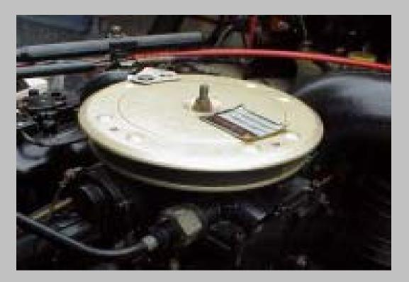
All gasoline powered inboard/outboard or inboard motor boats must be equipped with an approved backfire flame control device.
